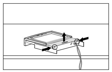
Figure 2-5. Removing the tray cover
